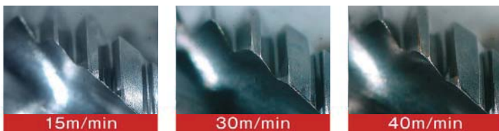
■ Cutting edge after 1.400 holes Tapping
