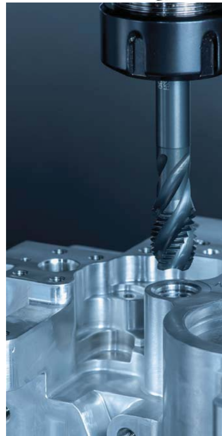
With its variable lead flute the A-SFT achieves optimized chip formation and evacuation.
